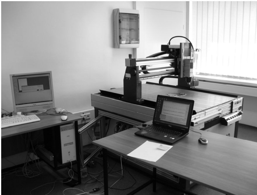
Fig. 5. Experimental test station with milling machine
