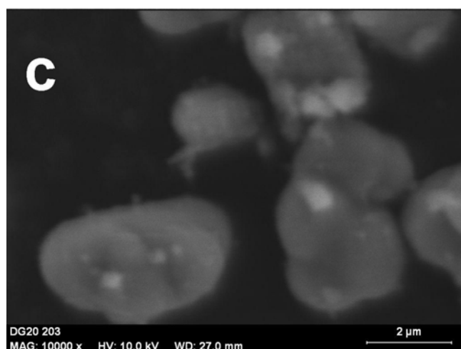
Figure 3. SEM images (magnification of \times 10000 ) of titanium dioxide obtained in the hydrolysis of titanyl sulphate using a) batch method and continuous method when the residence time the reaction mixture in the reactor was: b) 30 min, c) 60 min, d) 180 min. (the initial concentration of \text{TiOSO}_4 – 300 \text{ g/dm}^3 )
