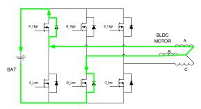
Fig. 6. Regenerative Current Flow for Step 1 of Commutation (Adapted from [10])
