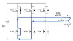
Fig. 5. Coasting Current Flow for First Commutation (Adapted from [10])
