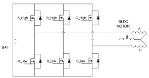
Fig. 2. Power Inverter Circuit (Adapted from [10])
