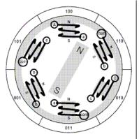
Fig. 1. Permanent Magnet BLDC Construction [4]
