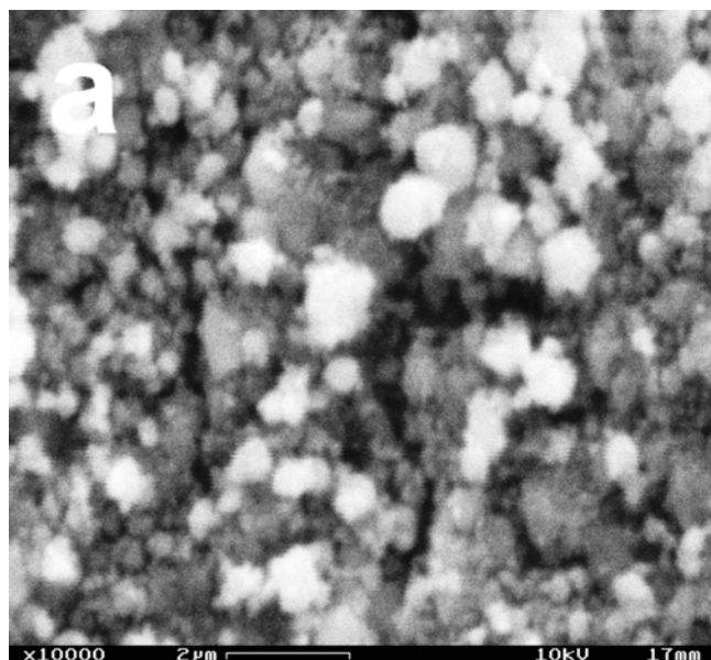
Figure 2. SEM images of titanium dioxide obtained in the hydrolysis of titanyl sulfate from a solution with the initial \text{Fe}^{2+} concentration equal to: a) 1.5 wt %, b) 5 wt %
