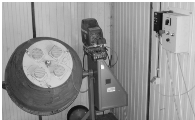
Figure 1. A rotational reactor with the air compressor and frequency converter
