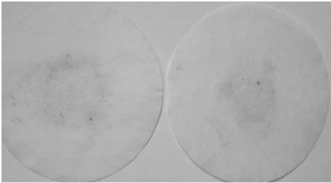
2%, pH 9, corrosion degree: 1
