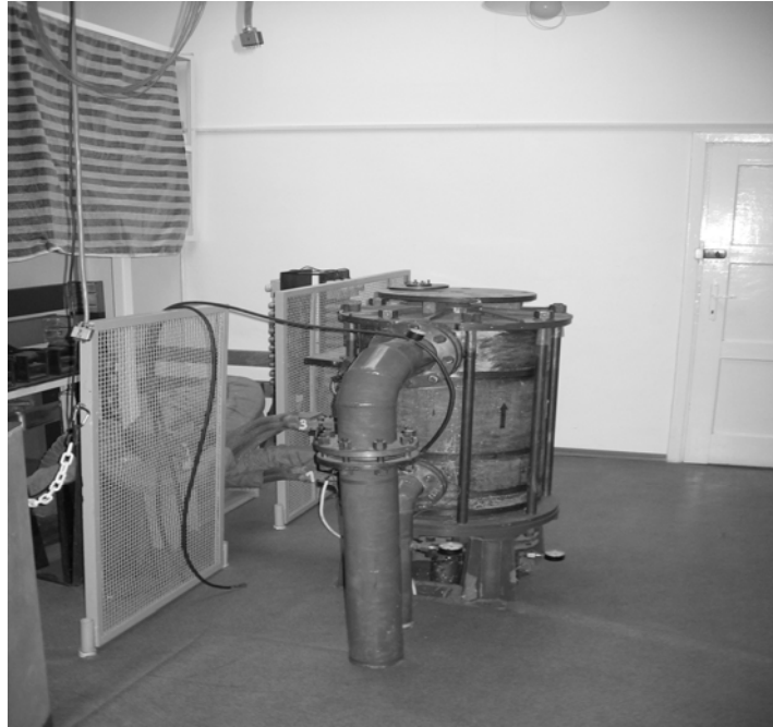
Fig. 2. View of the water cooled Bitter type electromagnet
