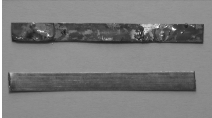
Fig. 9. Photograph of two pieces of HTc tapes: (up) deformed by applying bending strain and performing then the measurements, (down) straight nondeformed sample
