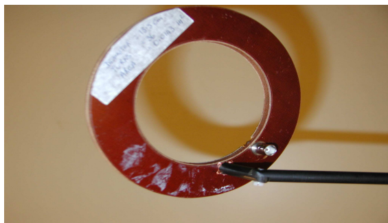
Figure 4. RE101 coil for measuring H-field emissions
