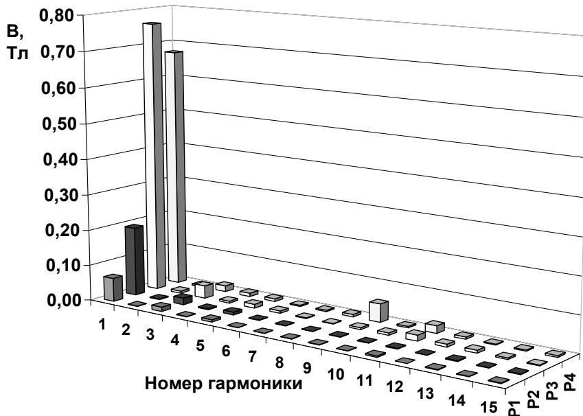
Fig. 9. Decomposition of normal and tangential components of an induction of a magnetic field in laminated ES stator the core in number Fourier on harmonious components. A number 1 (3) corresponds to decomposition of a normal (tangential) making induction in ES 1, 2, 3..., and a number 2 (4) – a normal (tangential) making induction in ES 42, 45, 48 ...
