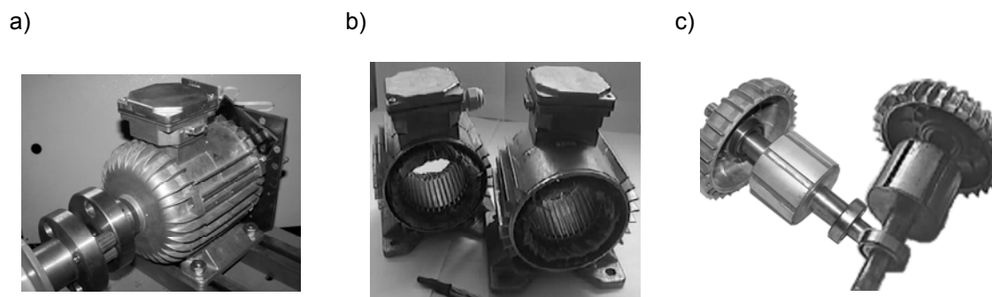
Fig. 1. Prototype of the motor (a), cores of stator with integral and fractional windings (b) and rotor with six poles and eight poles for an integral and fractional windings (c)
