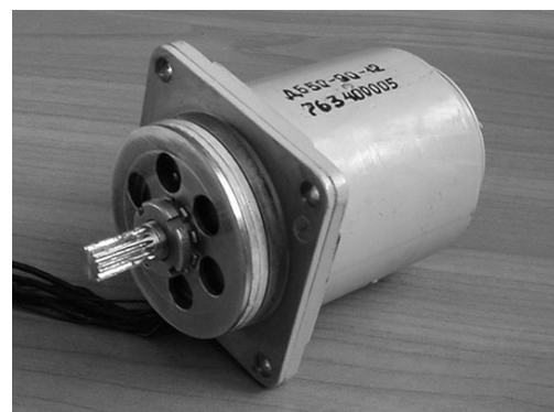
Fig. 2. The brushless DC electric motor DB50-90-8 of the aerodynamic control surface electric drive
