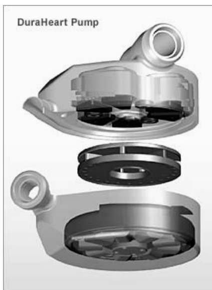
Fig. 6. Exploded view of DuraHeart® centrifugal rotary pump. Courtesy of Terumo Corporation, Tokyo, Japan
