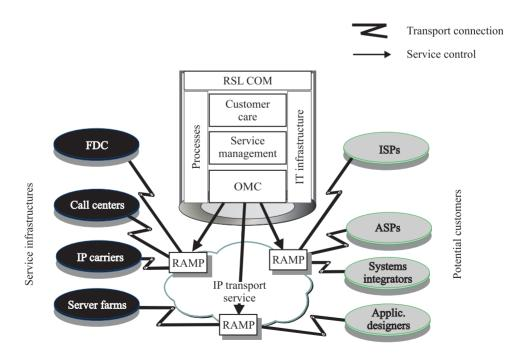
Fig. 15. Control of network and service
