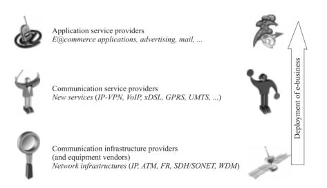
**Fig. 3.** Tiers of IP service value-chain ATM – Asynchronous Transfer Mode, FR – Frame Relay, IP – Internet Protocol, SDH – Synchronous Digital Hierarchy, VPN – Virtual Private Network
