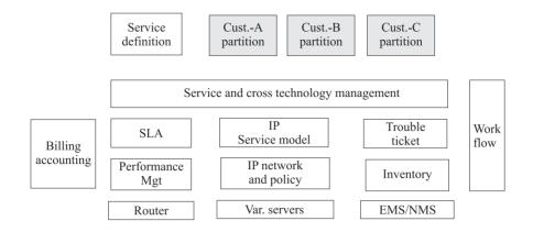
Fig. 10. OSS-architecture optimized for services
