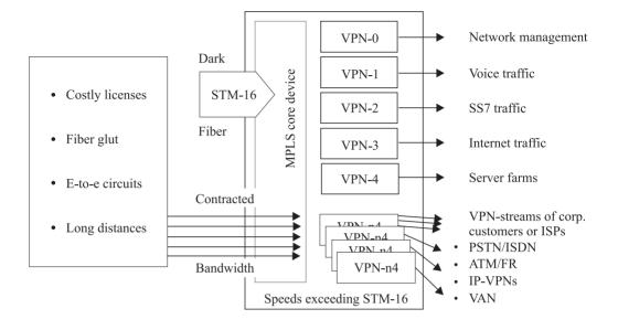
Fig. 5. MPLS – mapping VPNs to traffic streams
