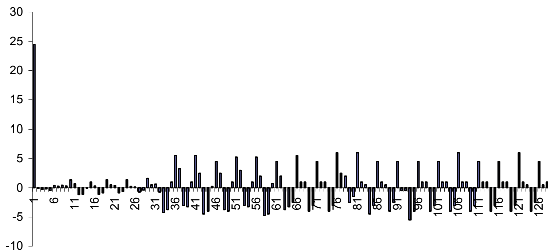
Fig.28. Current Haar spectrum for a faulty thyristor.
