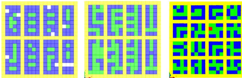
Fig. 12. Building structures shown in blue inside a preset grid of yellow coloured streets, the empty or free cells are shown in white or green. a) A block structure generated with R_2=7013 ; b) A structures with a lower density produced with R_3=5012 ; c) R_3 applied to a more fine-meshed grid of streets
