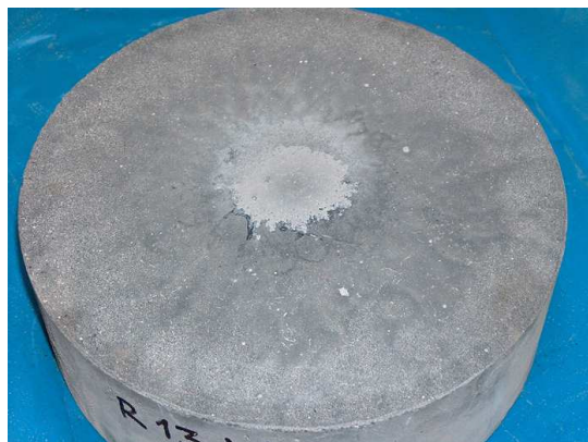
Fig. 5. Concrete specimen CF3 after 120 h of abrasion test (underwater method)
