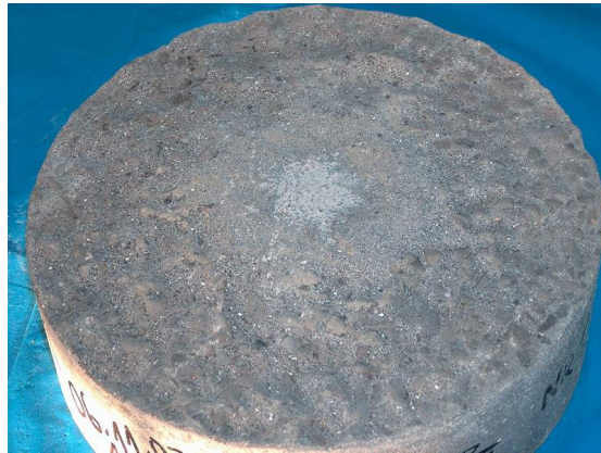
Fig. 4. Concrete specimen C0 after 120 h of abrasion test (underwater method)
