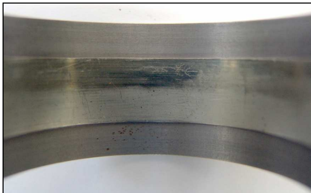
Fig. 4. Fatigue cracks of the SnCu6 surface layer after test on the MWO stand
