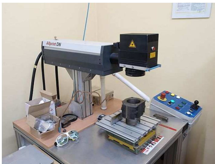
Rys. 4. Laser Nd: YAG Allprint DN ( \lambda = 1064 \text{ nm} , f = 100 \div 65 \text{ k Hz} , E = 50 \text{ J} , P = 50 \text{ W} )
