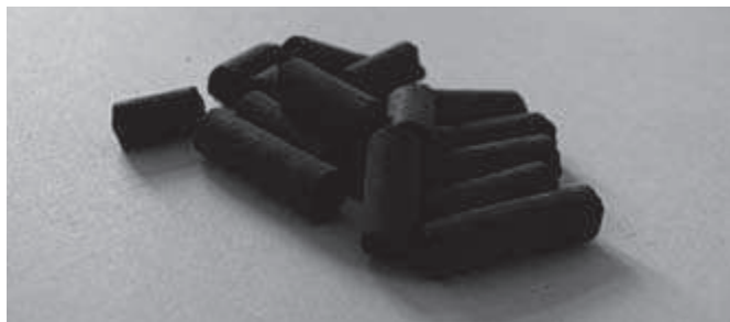
Fig. 6. Pellets from post-hydrolysis lignocellulose with 20.6% moisture content
