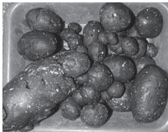
Fig. 4. The granulate obtained from the coal slurry provided by the Hard Coal Mine 'Piast' and produced with no admixture of a binding agent
