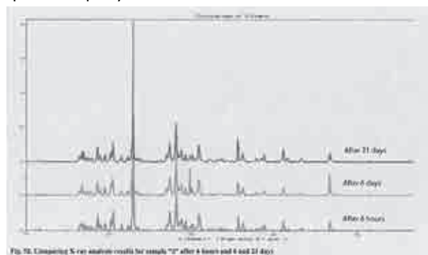
Fig. 6. Comparing the results of an X-ray analysis for the sample after 6 hours and 6 and 21 days
