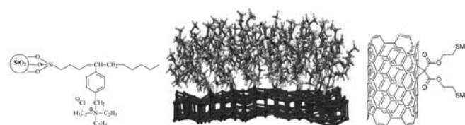
Fig. 2. Functionalized silica, metal surface and carbon nanotube
