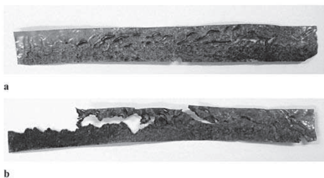
Fig. 2. Witness plates after detonation of nitro-chalk/aluminium powder mixtures in truncated cone 30÷45 mm: a – 97/3, b – 94/6
