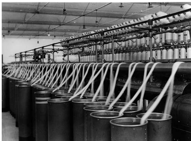
Arteks department; roving of short-cut fibres is subjected to throwing and wound onto coils
