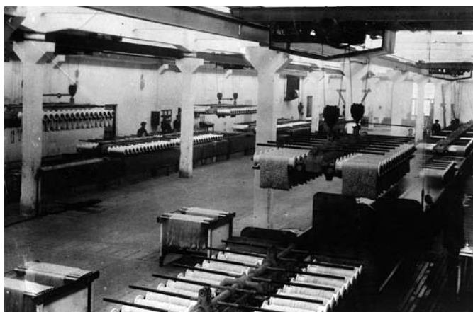
View onto the stripe finishing shop; silk in reels, after dyeing, is processed on Gerber machines
