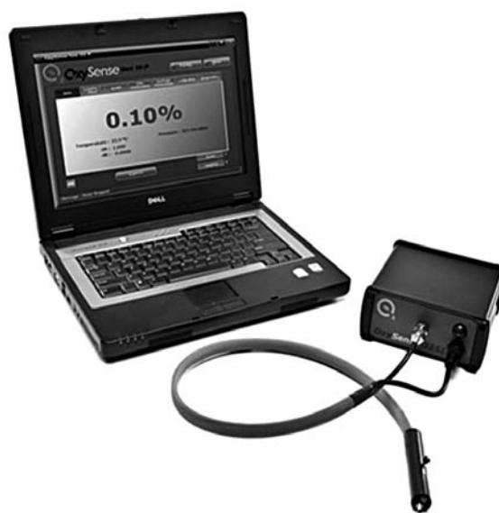
Fig. 1. The exemplary system for oxygen content measurement using the fluorescence phenomenon [2]
