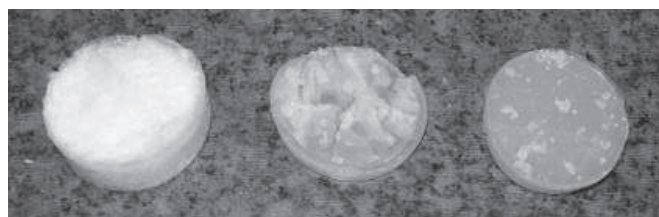
Fig. 2. A photograph of cracked biocatalyst blocks, prepared using sodium fluoride as catalyst at the following concentrations (from the left): 1 mol/dm 3 , 0.1 mol/dm 3 and 0.01 mol/dm 3
