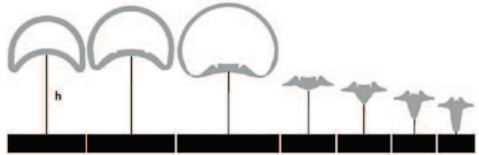
Fig. 3. The process of jet formation from the pressed shaped charge – time interval 3.00 \cdot 10^{-3} ms
