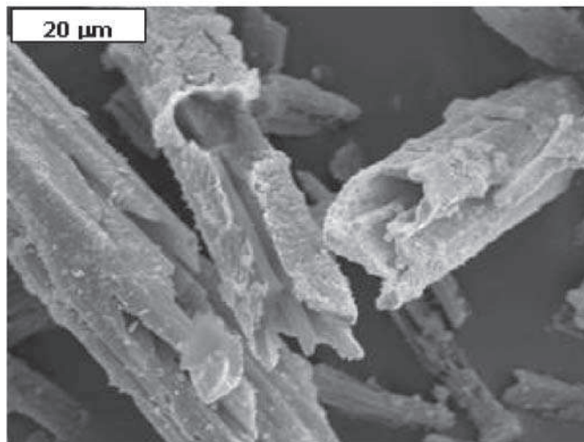
Fig. 5. Characteristic tubular-shape crystal forms of struvite produced in the presence of iron(III) ions. Process parameters: [\text{Fe}^{3+}]_{\text{RM}} = 0.001\% wt., pH = 10, \tau = 900 s, T = 298 K. Magnification: 1500x
