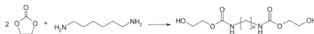
Scheme 7. Synthesis of the starter - 1,6-bis(2-hydroxyethoxycarbonylamino)hexane in the reaction of ethylene carbonate with 1,6-diaminohexane
