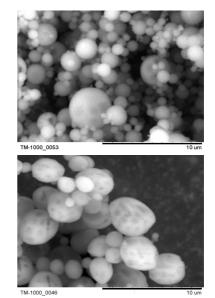
Fig. 2. SEM photographs of lactose particles (a) and lactose/biosurfactant particles (b)
