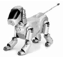
Fig. 2. Aibo dog-robot Sony company [4]
