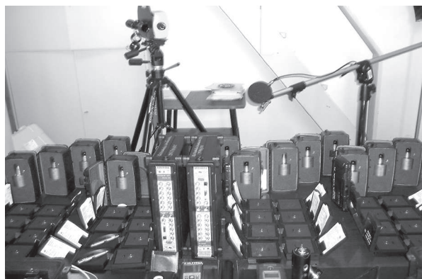
Fig. 1. Brüel & Kjær's PULSE system with 34 measure channels
