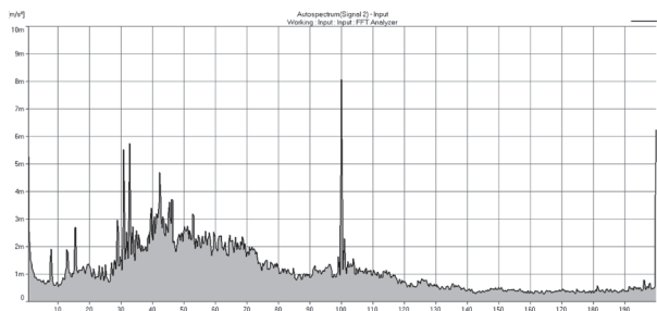
Fig. 6. Exemplary Autospectrum of accelerations (FFT analysis)
