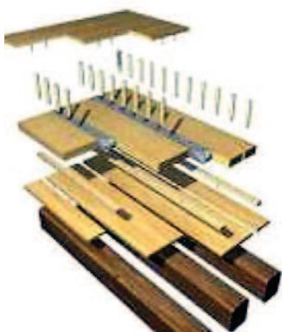
Fig. 17. Strengthening interventions, in and out of plane stiffening of an existing wooden floor: wooden planks at the extrados connected by wooden dowels
