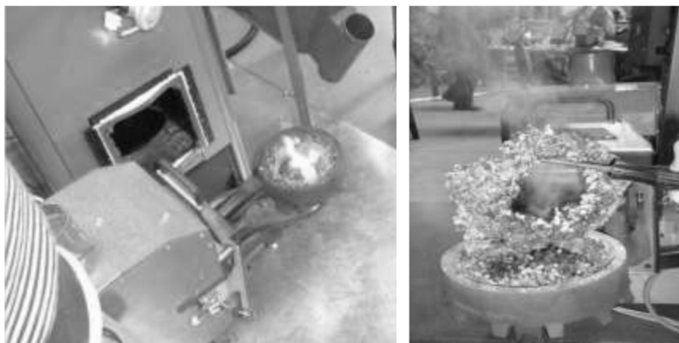
Fig. 3. Under-feed (retort) wood pellet furnace, slag can be observed during hay pellet combustion
