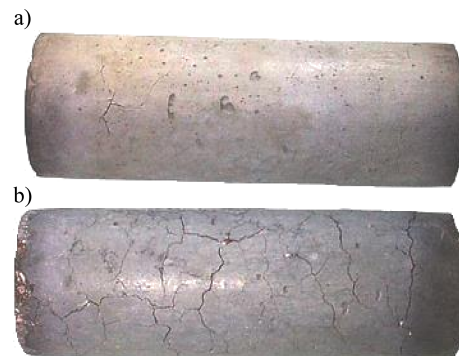
Fig. 7. Visible cracks on the surface of specimens after heating to 600°C, a) HPC with calcareous, and b) HPC with silico-calcareous aggregates
