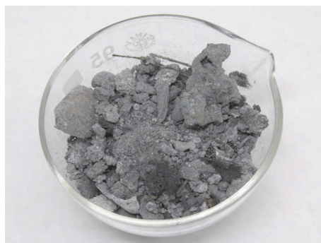
Fig. 1. Slag generated during the utilization of medical waste by Purotherm Pyrolyse technology
