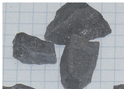
Fig. 2. The product obtained after the transformation of slag generated during pyrolysis of medical waste
