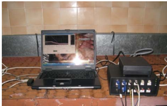
Fig.3. Measuring equipment: 1-computer, 2-multifunction data acquisition module Advantech USB-4711A, 3-converter PWM-2010.
