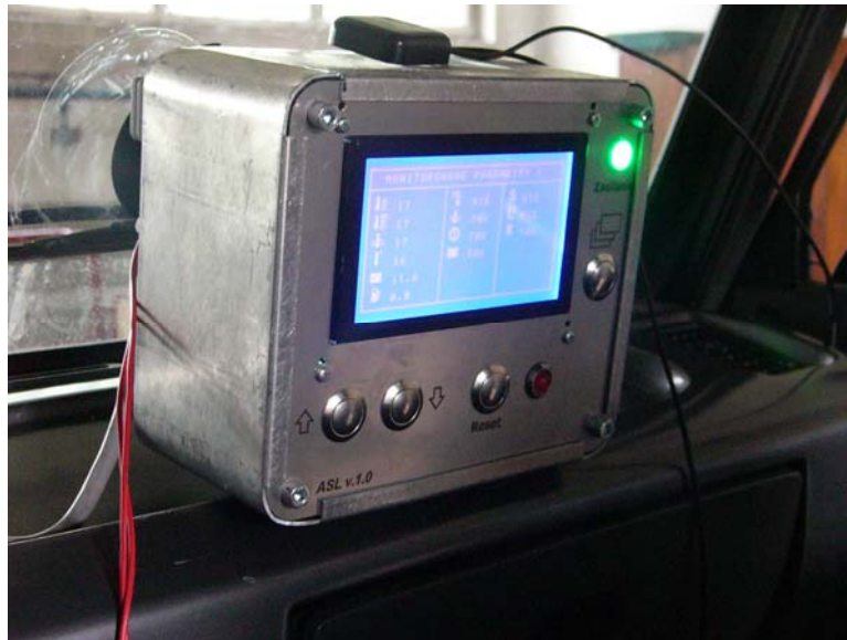
Fig. 4. View of the control panel in the prototype of the ALS v1.0 system (module No. 5)
