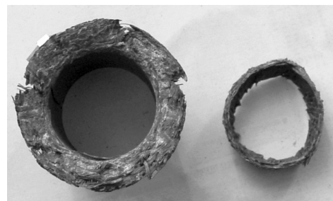
Fig. 9. C/E tube 73.4% filled with elastomer of 60°ShA
