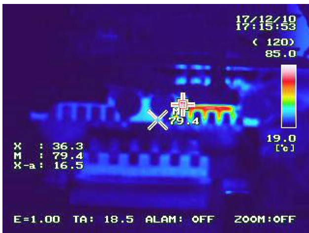
Fig. 14. Temperature distribution of the radiator, hard switching
