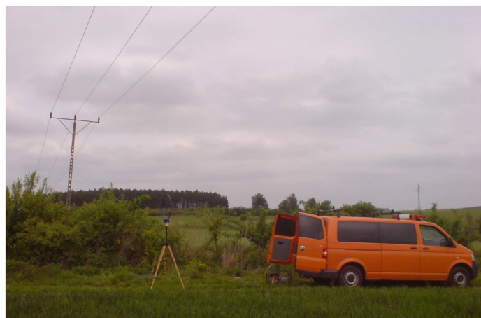
Fig. 14. Magnetic field measurement under overhead MV line
