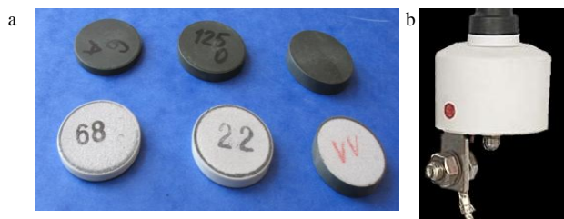
Fig. 2. Varistor specimens: a – structures after being fired (top) and with a metalized contacts (bottom); left – 280 V, middle – 440 V, right – 660 V; b - surge arrester with varistors.
