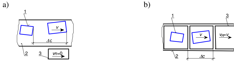
Fig. 2. Nonprehensile manipulators: a) stationary, b) stream; 1 – handled object, 2 – conveyor, 3 – working element of manipulator, v – velocity of load stream, v_R – velocity of manipulator, \Delta c – distance between heads of loads
