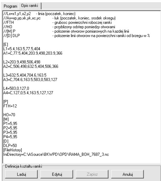
Fig. 9. Screen views for data entry and framework geometric features visualization a) input data describing the frame, b) frame drawing showing holes to drill location (green) and measuring points (red).
