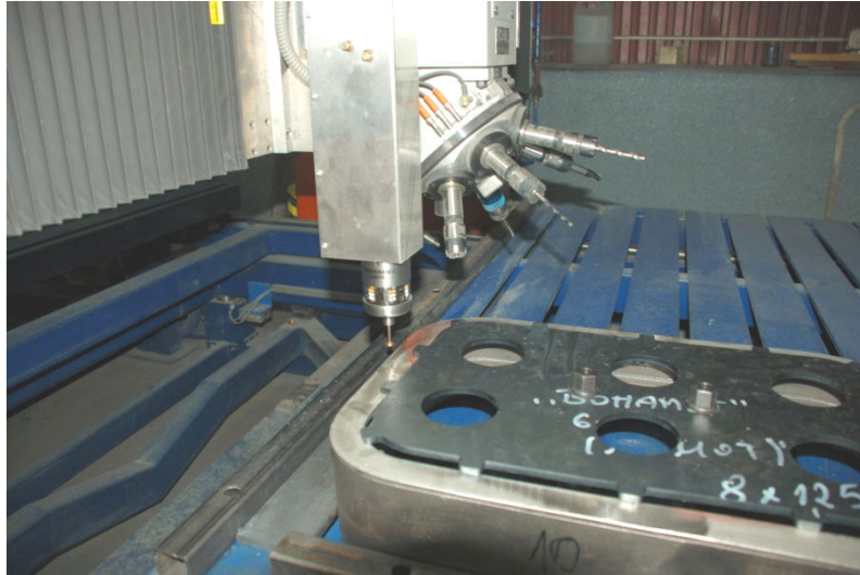
Fig. 6. Automatic measuring cycle of the ship frame
