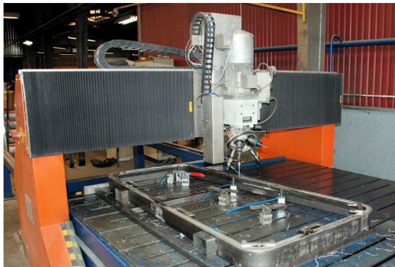
Fig. 5. View of drilling machine specialized for ship frames
