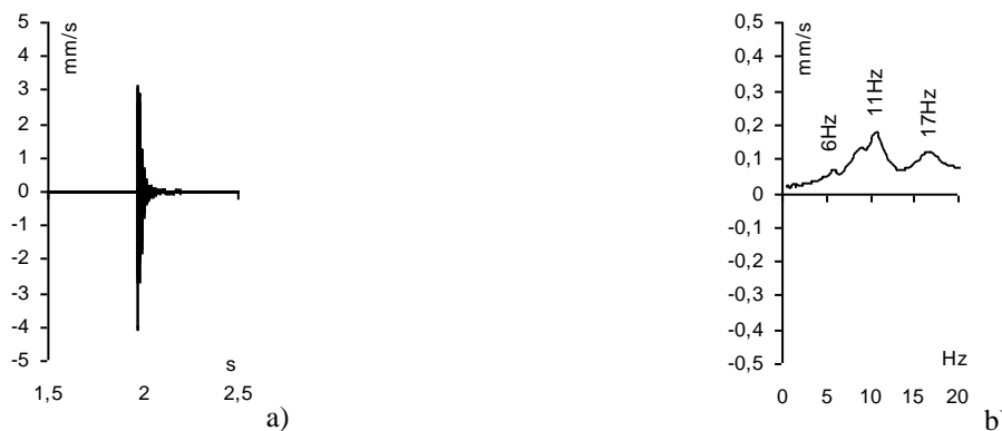
Fig.2.5. The response of the system to pulse induction: a) time course, b) characteristic A-C
