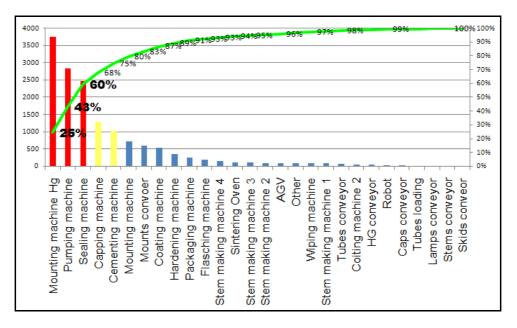
Fig.5. Time of breakdowns in min
