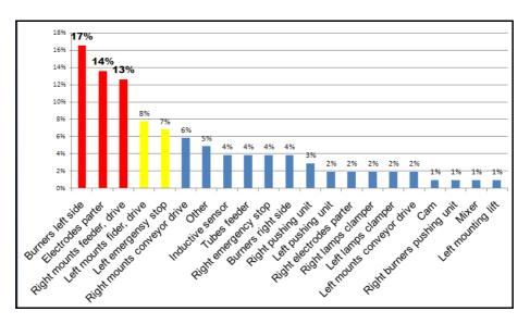
Fig.7. Breakdowns probability of sealing machines units
