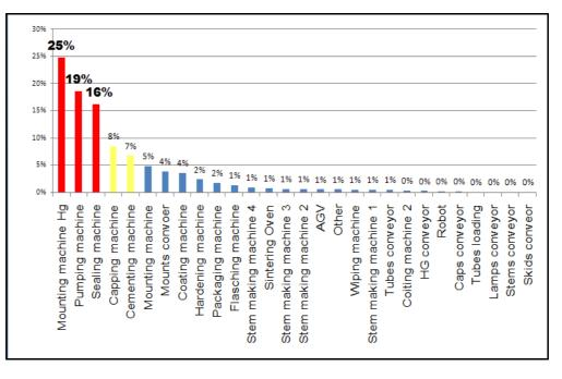
Fig.4. Probability of machines breakdowns
