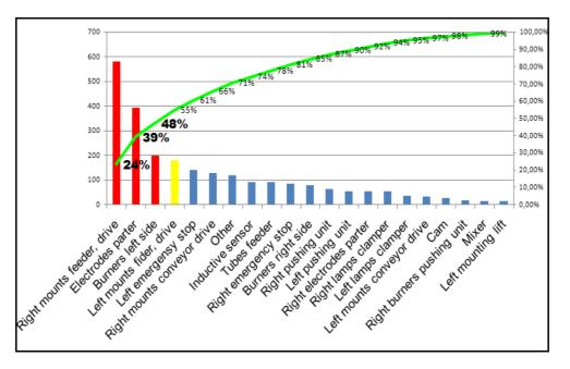
Fig.6. Breakdown time for sealing machine units
