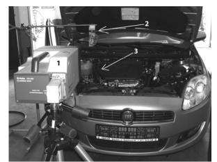
Fig. 2. Test rig: 1- laser probe, 2- mirror, 3- place of laser beam reflection
