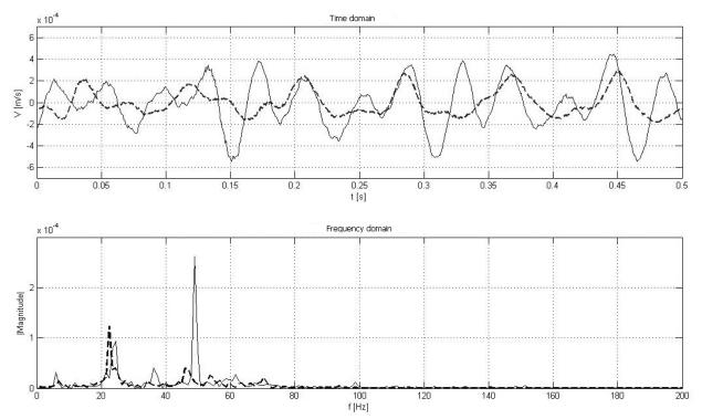
Fig. 4. Waveform and frequency spectrum of vibration velocities measured behind passenger handle for jacked up idle running car; solid line represents car having engine equipped with supercharger
