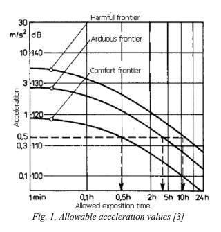
It is apparent from figure 1 that the comfort limit (the most representative quantity for the experimental results) is characterized by the lowest acceleration value which becomes extremely annoying after 10 hours. But this long journey by car is nothing extraordinary.
