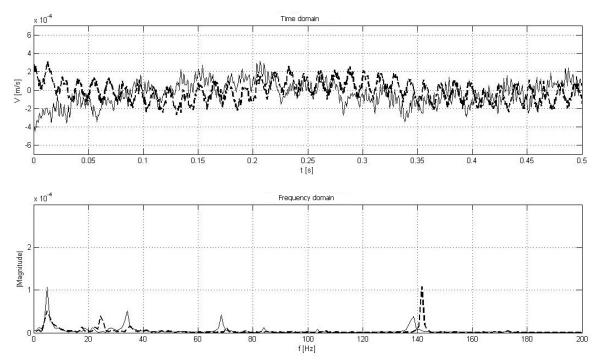
Fig. 5. Waveform and frequency spectrum of vibration velocities measured behind passenger handle for jacked up idle running (2000 rpm) car; solid line is for car having engine equipped with supercharger
