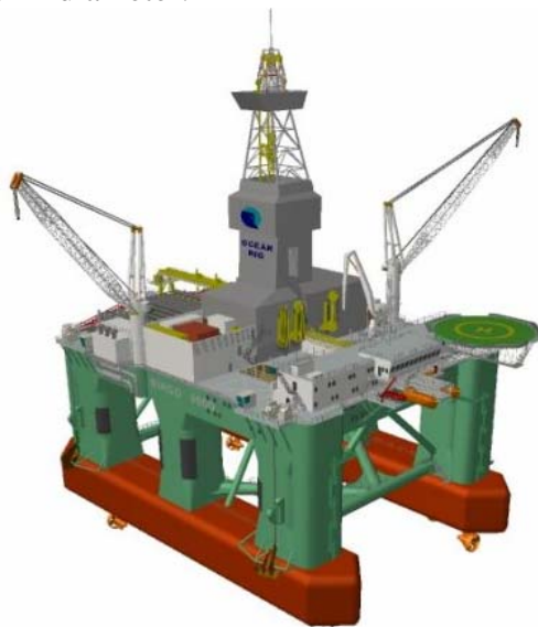
Fig. 14. Semisubmersible rig LEIV EIRIKSSON [1]
