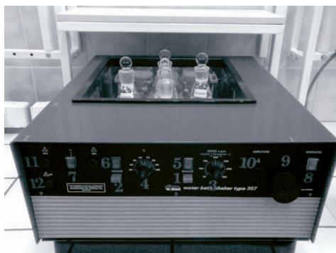
Photo 4. The set-up for determination of heavy metals sorption equilibrium
